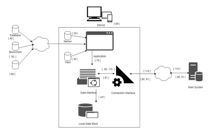
Figure 12 – Generating Data – It depicts an example of a system for collection of various kinds of data which is later used by a remote system for further processing.
